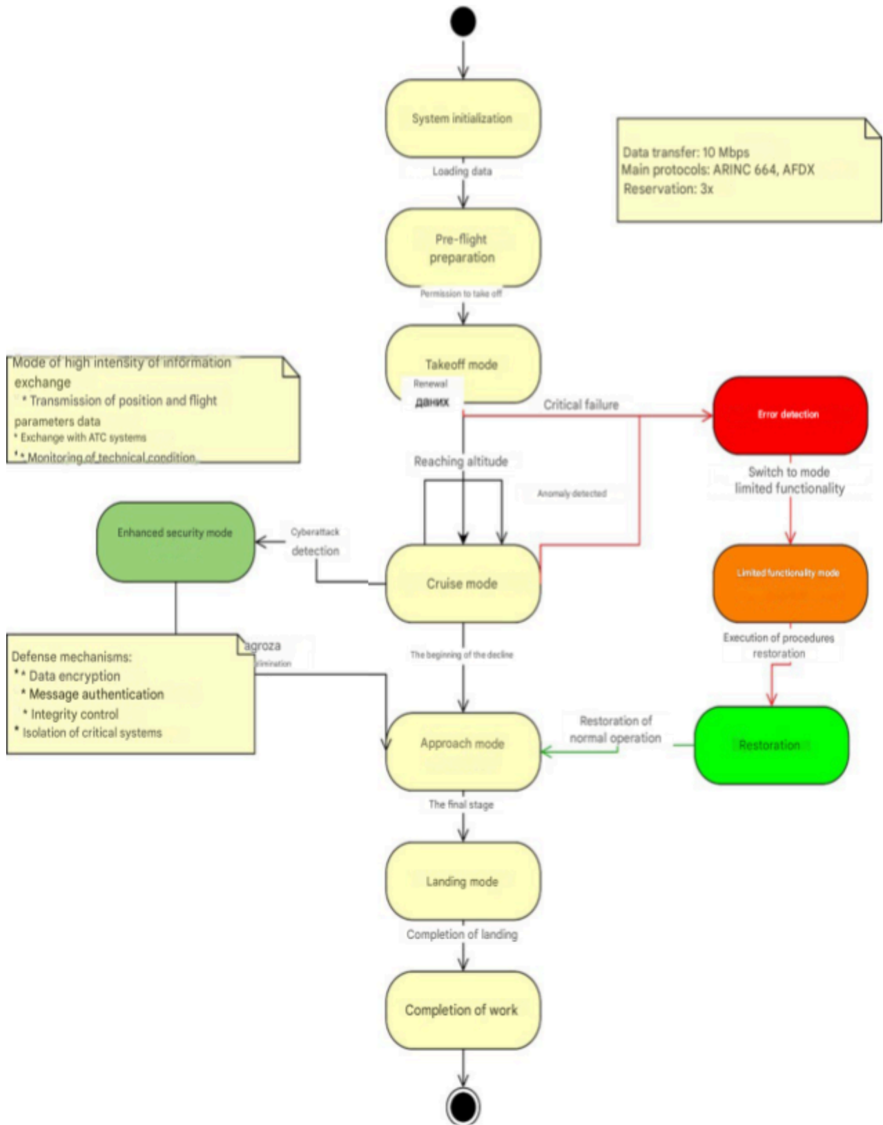
Fig. 3.1 - State diagram of the on-board information exchange system in different flight modes
